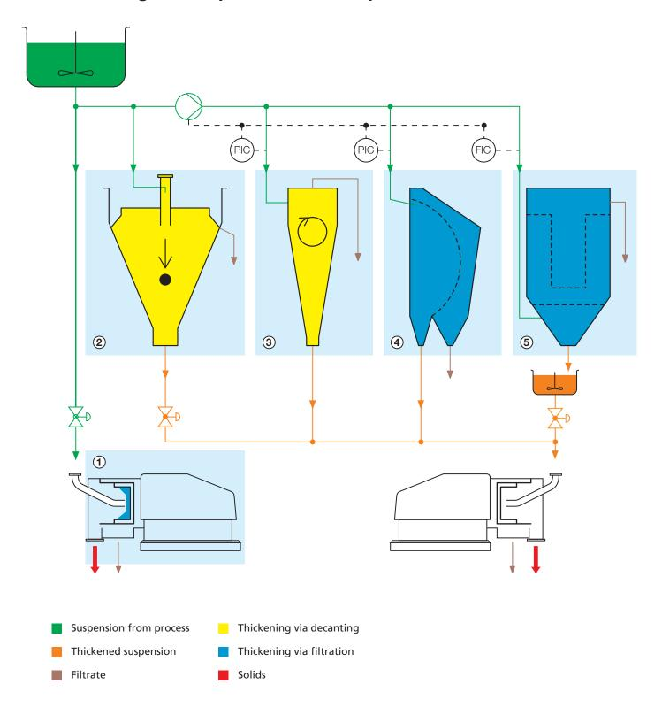
As a continuously operating machine, the pusher centrifuge requires process conditions and solids concentrations as constant as possible to ensure optimum operation and consistent product quality. For process and plant-related reasons, the necessary feed conditions are often not achieved. As a solution for this problem, Ferrum therefore offers various prethickening systems and dosing devices. Depending on requirements, Ferrum supplies the design, production and automation of the related system.
