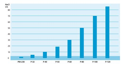
Maximum throughputs of Ferrum pusher centrifuges with NaCl (throughputs dependent on feed conditions)
