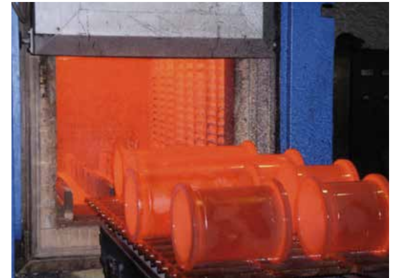
Fig. 4: Components in front of the furnace after completion of the firing operation. Homogeneous temperature distribution within the component is the basic requirement to ensure quality enamelling.
