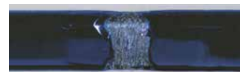
Distension reduced failure picture of enamel in the bending test in the area of the plastic deformation (load transmission). Outside of the plastic zone, left and right, damage-free enamel.
