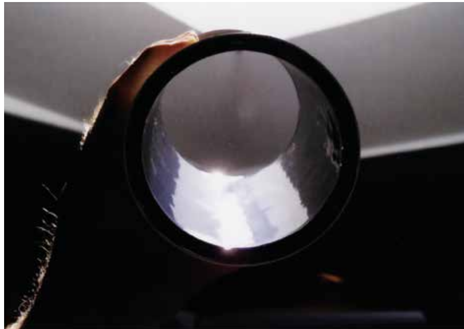
Fig. 1: Industrial enamel with extremely smooth surface finish in conjunction with high wear resistance to abrasive acting media and high resistance to corrosion. Visual counter light inspection of surface.
